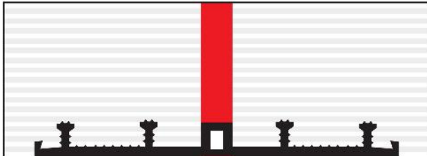
Expansion joint waterstops, external
